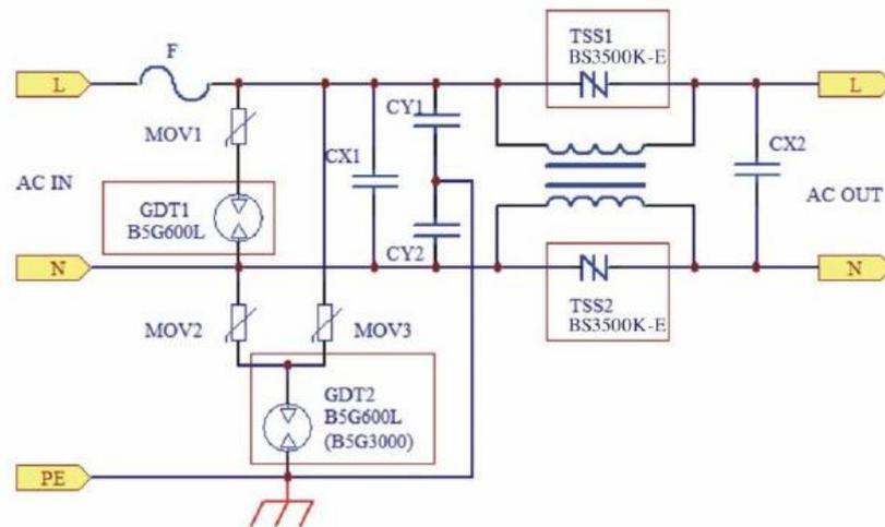
Figure 2 The main electrical protection measures
